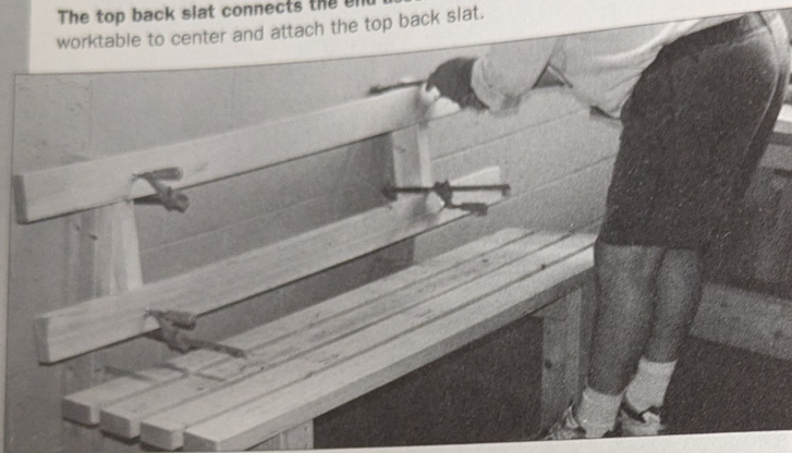
Complete the back. Glue and screw the bottom back slat to the sloper.
